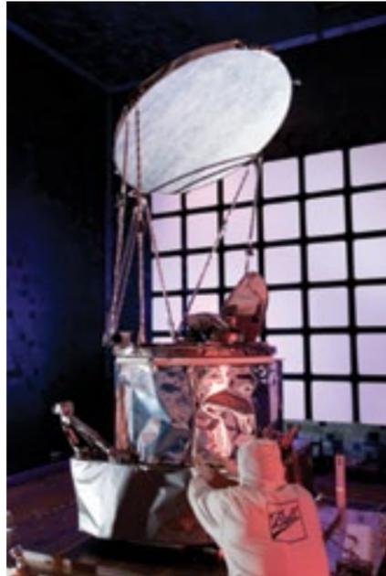
**Ball-built Global Precipitation Measurement (GPM) Microwave Imager (GMI) in a Ball Aerospace clean room prior to shipment to Goddard Space Flight Center for integration with the spacecraft. Image: Ball Aerospace**
